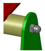
Adding another Cap Nut Holding down Ctrl drag another cap nut from the feature manager design tree. Rotate the cap nut to the orientation
