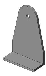
**Extruded Boss/Base Extrude** the sketch using the Blind End Condition and a Depth of 20mm
