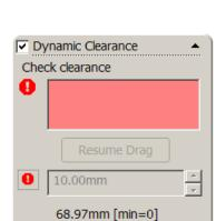
**Dynamic Clearance** You can dynamically detect the clearance between components when moving or rotating a component. As you move or rotate a component, a dimension appears indicating the minimum distance between the selected components.
