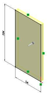
The edge of this extrude is inclined so we must select the draft button and set it to 3 degrees. Set the distance to 5.5mm as shown in the dialog box.
