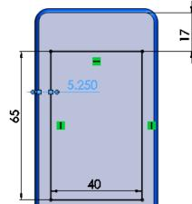
The next step is to create the lower section where the buttons are situated. Open a sketch on the same plane. Sketch and dimension this lower section like the sketch displays.
