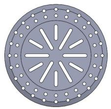
The advantage of this method is that changes can easily be made to the instances either by selecting them on the design tree or on the screen.
