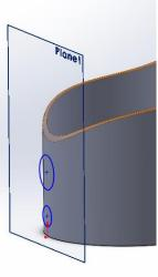
Now highlight inside face and delete face and accept.... this will effectively remove the inside skin... now remove the remaining walls...
