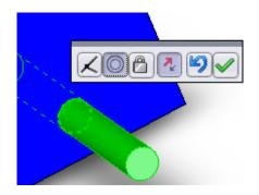
A new dialogue box appears on the screen as can be seen Above. This box allows you to change the mate used or to Confirm the selected mate with the OK button.
