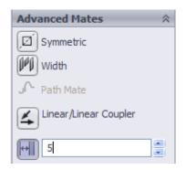
The end of the axle will now move to Within **5mm** of the car body as shown.
