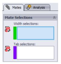
The box marked Width selection Will contain the surface from which You wish to set the distance from, in This case the **Car Body.** Left click The car body as shown to select it
