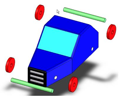
**Introducing Mates:** Mates are used in assemblies to join components together.
