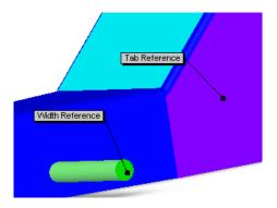
Finally select the distance button in advanced mates, as before, and set the distance to **5mm**.
