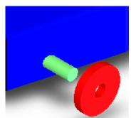
To finish this mate select the outside Surface of the wheel, as shown
