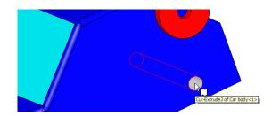
Solidworks will now automatically make the Axle and the axle hole Concentric as shown.
